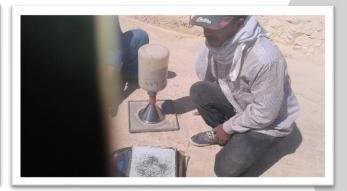
**Test for soil compaction**
