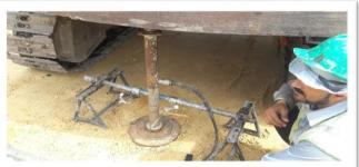
**Plate Load Test on Soil Replacement**
